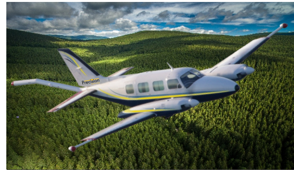
Precision's 3-sensor fixed-wing system provides economical 2-axis gradient data suitable for gentle terrain.
