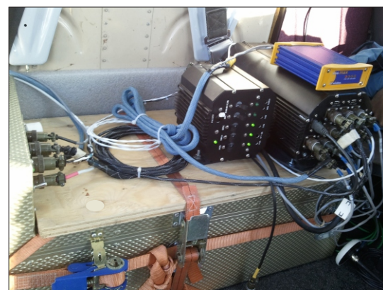
Spectrometer crystals installed in AS350 survey helicopter
