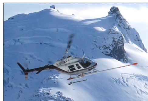
High resolution single-sensor magnetic survey by helicopter
