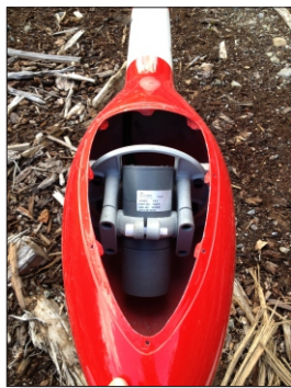
Stinger-mounted mag sensor
