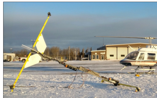
Precision's unique 4-sensor gradient system provides 3-axis data under a helicopter. Best suited for gentle to moderate terrain.
