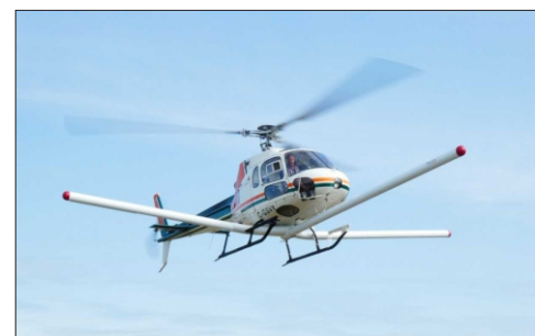
Multi-sensor (gradient) helicopter survey
