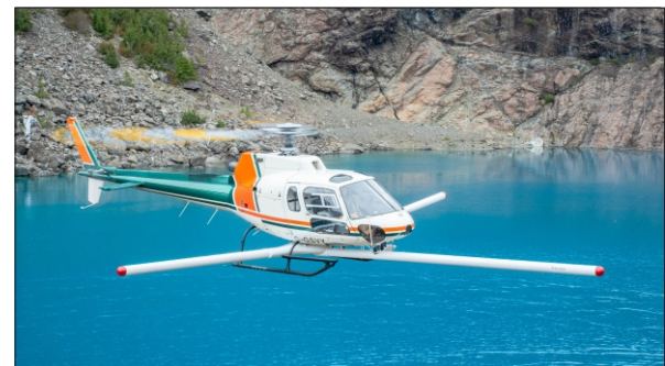
Precision's helicopter-mounted 3-sensor system provides 2-axis gradient data in steep terrain.
