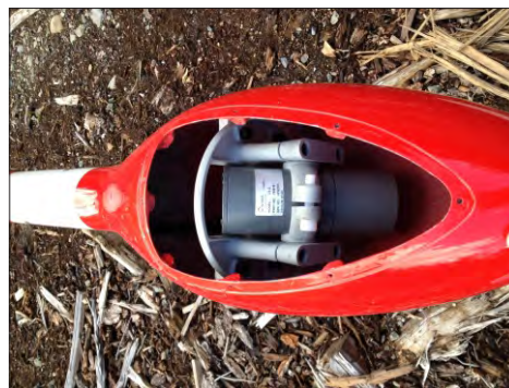
Stinger-mounted mag sensor
