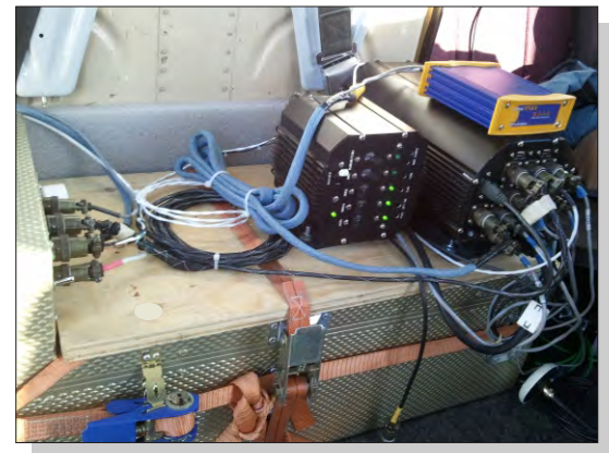
Spectrometer crystals installed in AS350 survey helicopter
